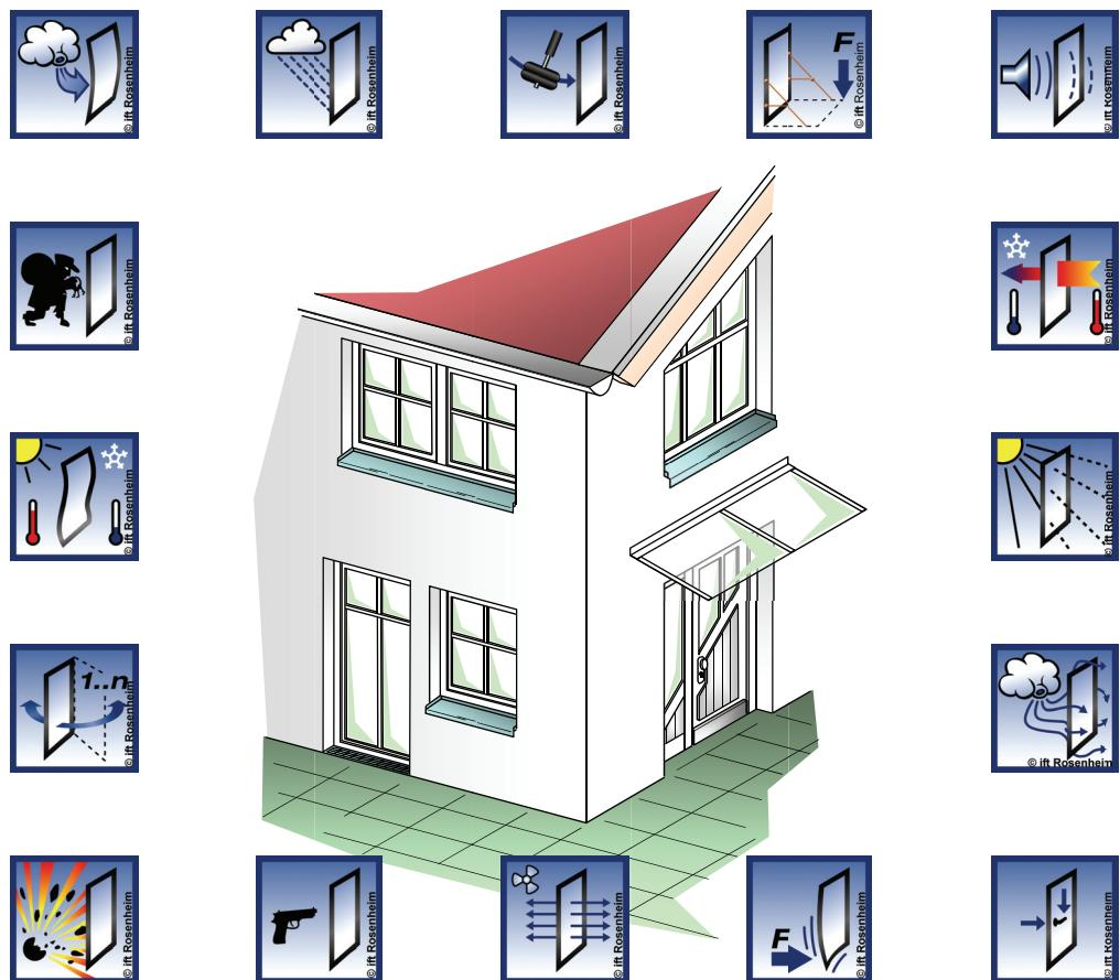
**Figure 2.1** Windows and exterior doors as multifunctional building components, selected properties in accordance with Product Standard EN 14351-1
